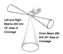
Wide Side is an accessory transducer that gives your Wide 3D Vista the capability of collecting sonar information from either side of your boat. Side-looking sonar is extremely valuable for bank fishing, or looking for bait fish in open water.
